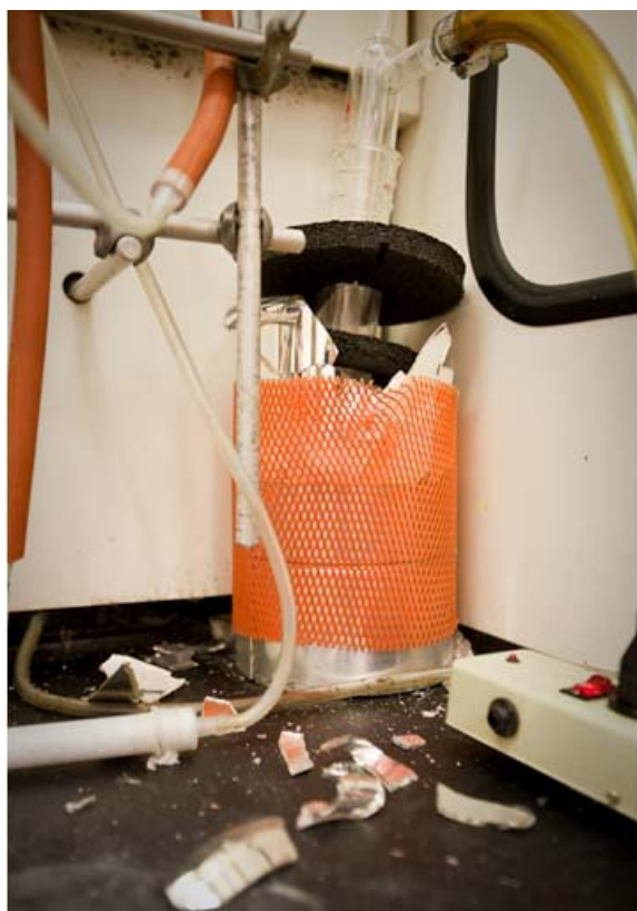
Exploded Dewar flask with original protective plastic mesh after explosion.
