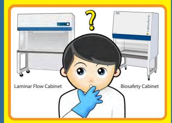
Laminar flow cabinets can look very similar to biosafety cabinets, but they only protect samples inside the work zone from external airborne contamination. They do not protect the operator. Read the labeling on your cabinet carefully before proceeding.
