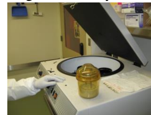
Sealable aerosol-tight secondary containers for centrifuge
