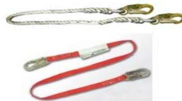
**Connectors:** A device, which is used to connect parts of the personal fall restraint system together. It may be an independent component of the system, such as a carabiner, or it may be an integral component of part of the system (such as a d-ring sewn into a harness, or a snap-hook spliced or sewn to a lanyard). All connectors must have locking features to avoid unclipping.
