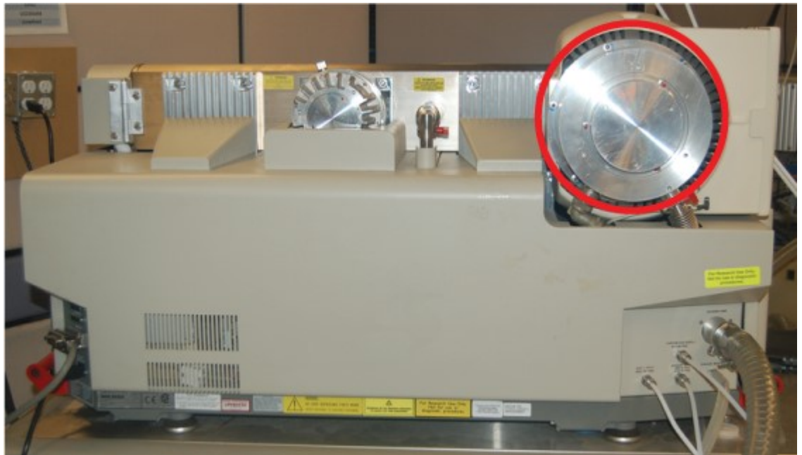
Figure 1: Turbo Pump (Shown Inside the Red Circle)
