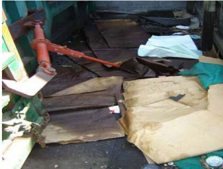
Hydraulic Leak from dumpster
